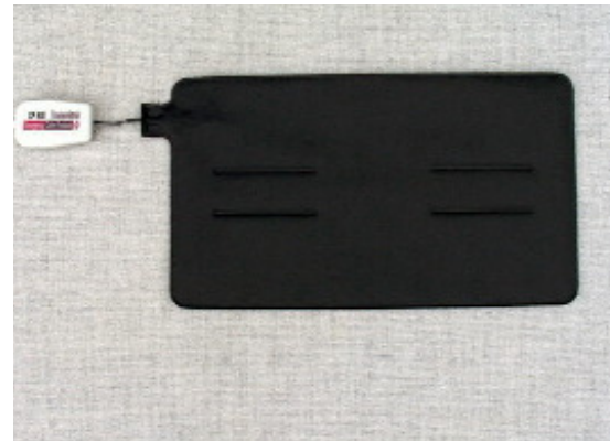
XP-3-300 Transmitter sensor pad should be tested at least once per week.
